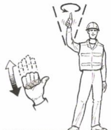
Inch load Clench and unclench fingers to signal 'inch the load'
